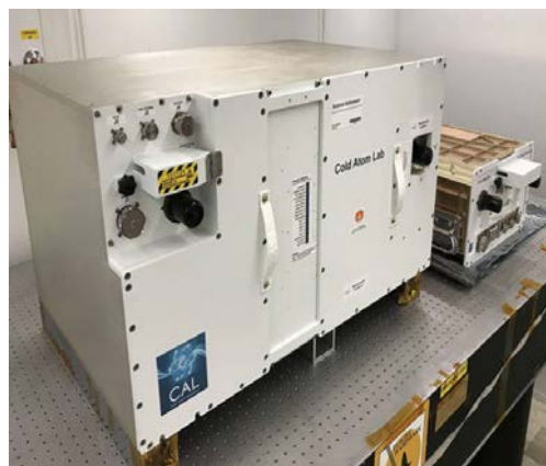
COLD ATOM LAB. About the size of a mini fridge, the Cold Atom Lab Science Instrument (left) contains the Science Module, which cools atoms to nearly absolute zero. The smaller box on the right contains additional hardware. (Credits: NASA/JPL-Caltech)
