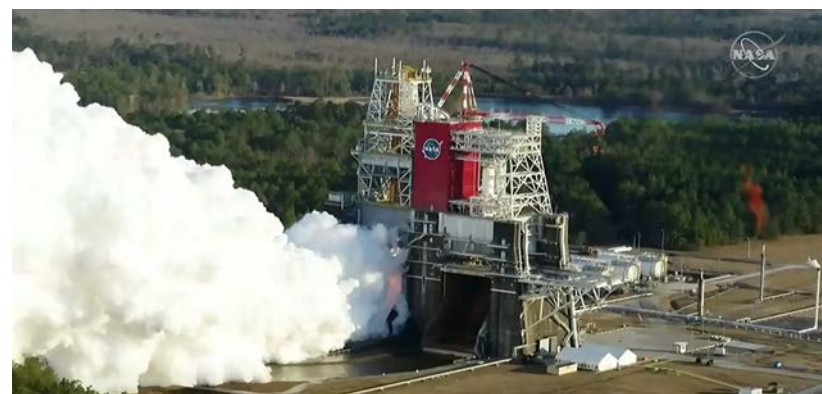
The core stage for the first flight of NASA's Space Launch System rocket is seen in the B-2 Test Stand during a hot fire test Jan. 16, 2021, at NASA's Stennis Space Center near Bay St. Louis, Mississippi. (Credits: NASA Television)
