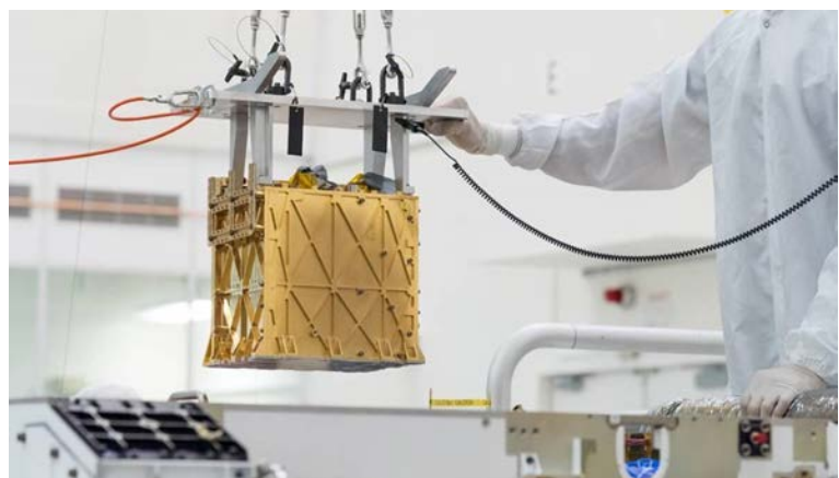
Technicians at NASA's Jet Propulsion Laboratory lower the Mars Oxygen In-Situ Resource Utilization Experiment (MOXIE) instrument into the belly of the Perseverance rover. (Photo: NASA/JPL-Caltech)
